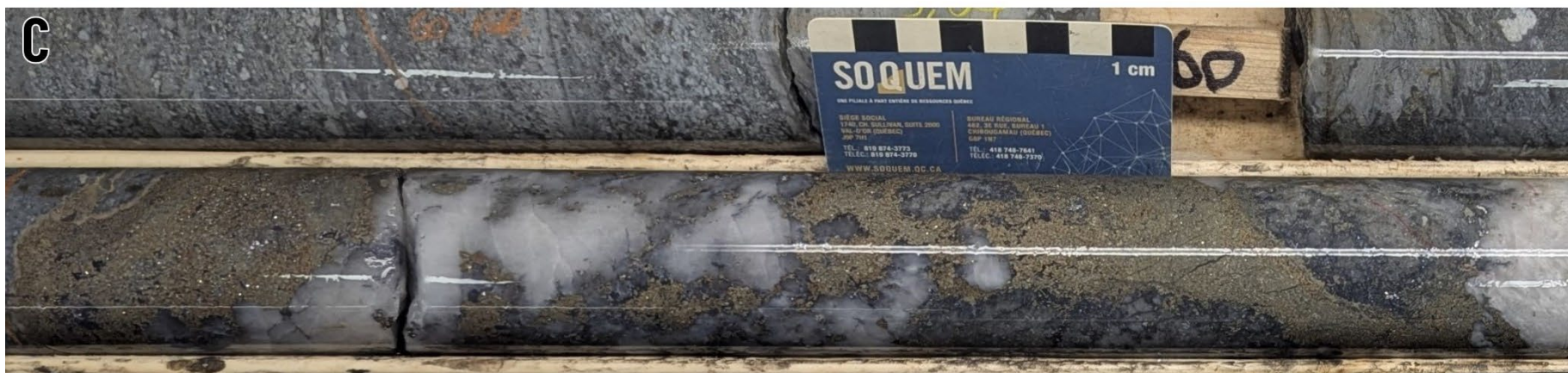
Figure 7. Different types of mineralization intersected in the Silver 2 Zone. Photo A shows mainly pyritic mineralization, locally with sphalerite, galena and native silver, near the exhalative contact within the favourable stratigraphy in hole 1338-26-100. Photo B shows a cluster of native silver in the same interval described in "A". Photo C shows the second type of mineralization encountered in the Silver 2 Zone (hole 1338-26-102): quartz and sulphide injections.
